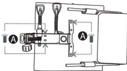
**5. Place the seat with the hole in the adjusting mechanism onto the gas lift**
